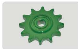
G52776 OEM No.: AA32776 Weight: 0.35 lbs 12 tooth Idler sprocket for 50 chain. For use on seed transmission, also drive wheels on John Deere planters 7200, 7300, 7340, 1700, 1705, 1710, 1715, 1720, 1725, 1730, 1735, 1750, 1755, 1770, 1770NT, 1775NT, 1790, 1795, DB series. Bore size 1/2".
