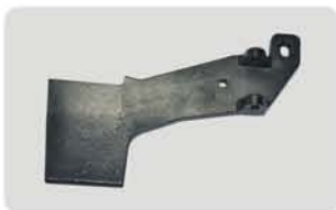
G52157 OEM No.: A52157 Weight: 5.73 lbs Liquid single disc fertilizer cast shoe, LEFT Hand. Used on John Deere single disc openers mounted to 3"x3", 3"x7" or 5"x7" fertilizer bars; also 6"x10" or 7"x7" bars prior to s/n 720100.
